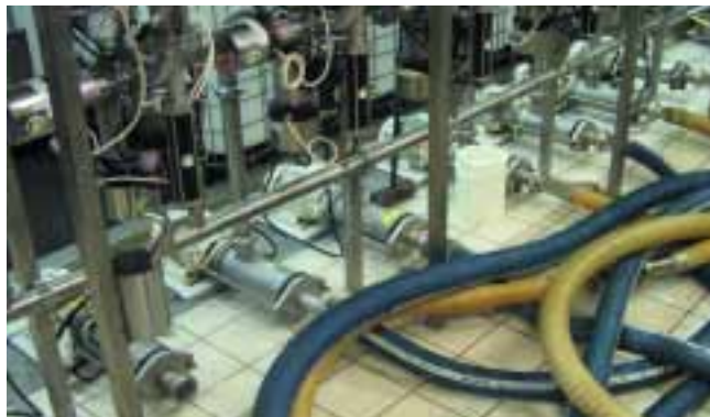
Compact M6000C4 for the transfer of soap base in the cosmetic industry.
